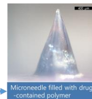
Microneedle filled with drug-contained polymer
